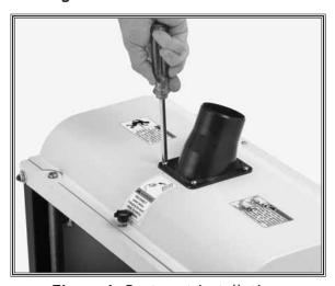
Figure 6. Dust port installation.
